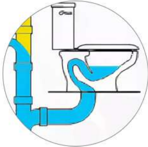
Soil pipe from a toilet - 4"
