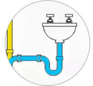
Drain pipe from hand basins - 1 1/4"
