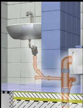
Keep the drain as short as possible
